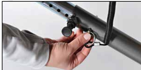
Ensure safety pin is always left inserted after every adjustment is made
